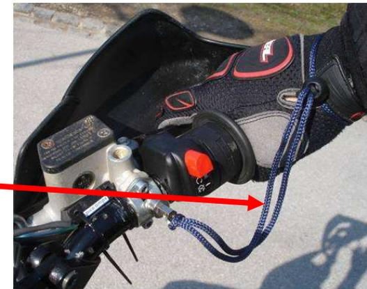
**WARNING!** The iron parts of the anchor point may themselves become magnetic after some time and as a consequence obstruct that the magnetic switch opens when pulling off the magnet. In this case the magnetic switch has to be repositioned as described above so that it opens reliably.
