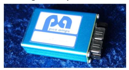
Using the picoamps DMMD your e-bike will react like a gas bike. In combination with the picoamps SENS-50 current sensor a digital microprocessor controls the motor current and thus the torque with respect to the throttle opening. The response characteristics of the module can easily be adapted to the special needs of the driver by selecting software parameters.
