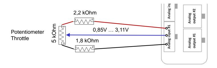
Using a DMMD configured for Potentiometer type throttle, the configuration of the DMMD software has to be changed for a conversion from **Potentiometer to Hall type throttle.**
